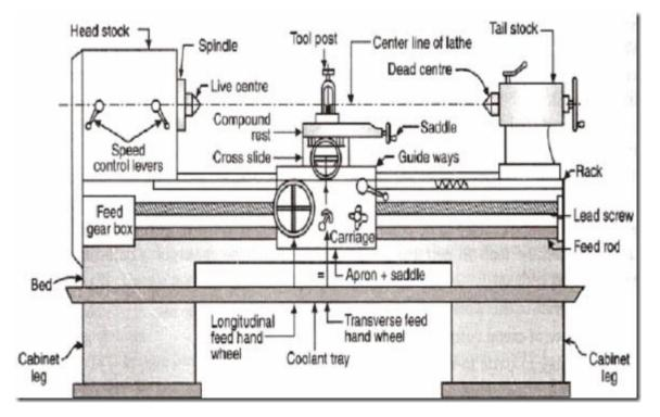
1. **Bed**: The bed is a heavy, rugged casting in which are mounted the working parts of the lathe. It carries the headstock and tail stock for supporting the workpiece and provides a base for the movement of carriage assembly which carries the tool.
