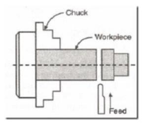
4. **Parting**: The parting or cutting off is the operation of cutting away a desired length of the workpiece, *i.e.*, dividing the workpiece in two or more parts.
