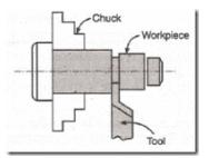
10. **Threading**: Threading is the act of cutting of the required form of threads on the internal or external cylindrical surfaces.
