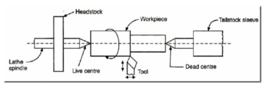
**<u>Construction</u>**: The main parts of the lathe are the bed, headstock, quick changing gear box, carriage and tailstock.
